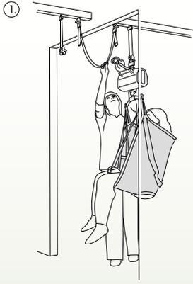
Attach the Strap Gripper to the Room-to-Room Strap and lower the lift. The patient's weight is gradually transferred to the Room-to-Room Strap.
