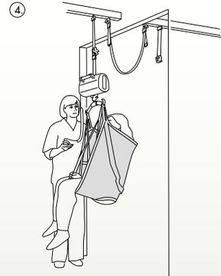
When the patient has been transferred to room 2 completely, the Strap Gripper is removed from the Room-to-Room Strap and the transfer along the rail can continue.
